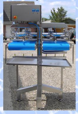
Easy Matic pinbone remover is designed to remove as many pinbones as possible without damaging the fillet, and thereby lowering the waste.
